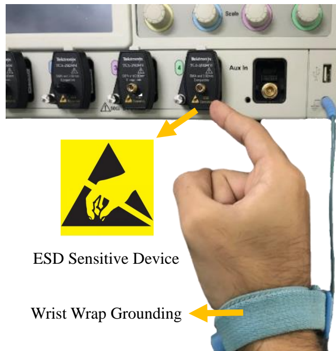
Figure 59 – DPO with ESD sensitive inputs. The wrist wrap grounds the user, protecting the equipment from ESD.
