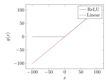
Figure 3 – Rectified Linear Units vs. Linear Units.
