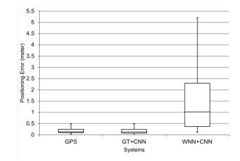
Figure 27 – Comparison between hybrid WNN-CNN system and GPS positioning error.
