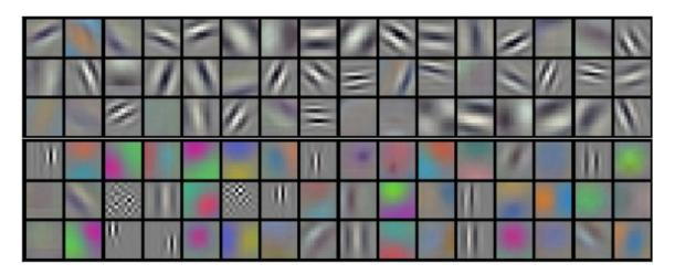
Figure 4 – Filters learned by first convolutional layer of AlexNet (KRIZHEVSKY; SUTSKEVER; HINTON, 2012). Each of the 96 filters has size 11 × 11 × 3 and the input image size is 224 × 224 × 3. The top three filter rows were learned on a GPU while the bottom three filter rows were learned on another. Figure courtesy of (KRIZHEVSKY; SUTSKEVER; HINTON, 2012)
