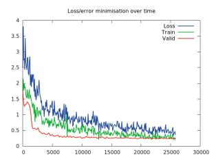
Figure 23 – Network training evolution. The vertical axis represents the error in meters and the horizontal axis represents the training iterations. The curves in indigo, green and red represents the error measured in meters of the loss function, training and validation data.
