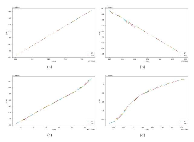
Figure 24 – Performance of GPS-RTK Trimble on UFES-LAP-09-LAP-09-5m-1m test dataset. Each sub-figure represents a sequence of 50 points randomly selected from UFES-LAP-09-LAP-09-5m-1m test dataset. Green dots represents the ground truth while the red dots represent GPS coordinates. Connecting the corresponding ground truth and GPS dots are varied-colored lines.
