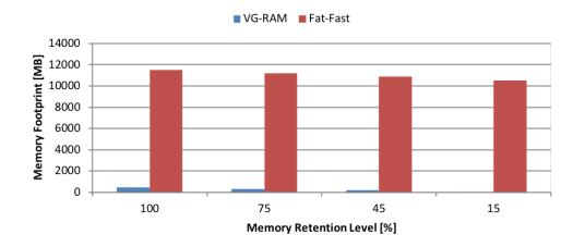
Figure 21 – Memory footprint of the Place Recognition System implemented with standard VG-RAM neuron, and Fat-Fast neuron with p/h = 16 bits and r = 30.
