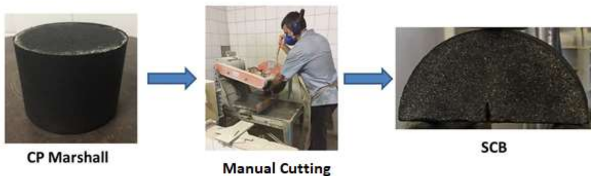
FIGURE 25 – ACTUAL SCB SPECIMEN CORING AND CUTTING PROCEDURE
