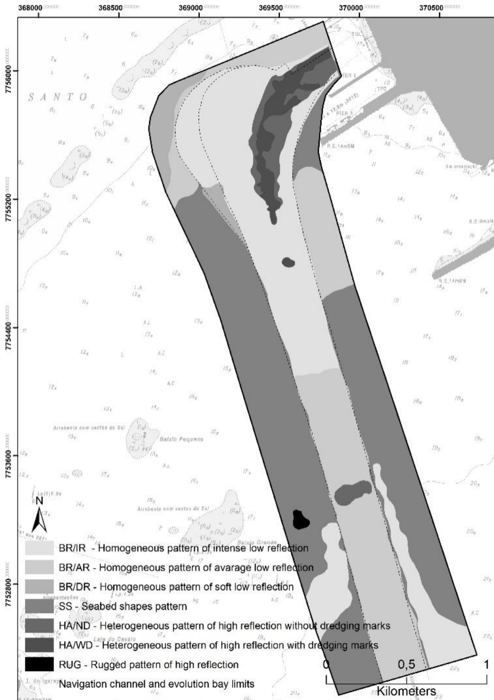
Figure 10 - SSS backscatter pattern compartmentation.
