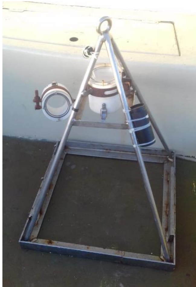
Figure 3 Drop-camera system used to acquire ground truth data. Two GoPros and two flashlights are attached in the metallic structure to record videos of the seafloor
