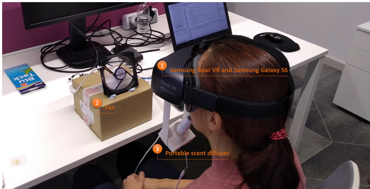
Figure 17 – A 360° VR mulsemmedia system that includes audiovisual content displayed on an HMD integrated with a fan and a portable scent diffuser.
