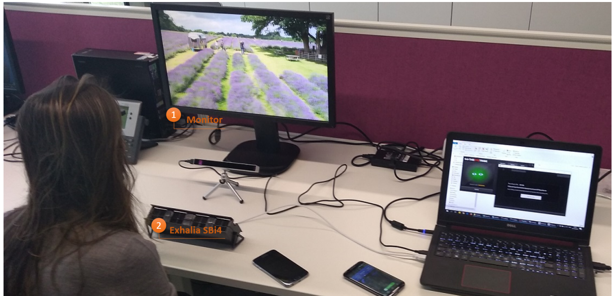
Figure 16 – Smell-intensive system—audiovisual content along with scent delivered through four emitters at the same time using USB connectivity.
