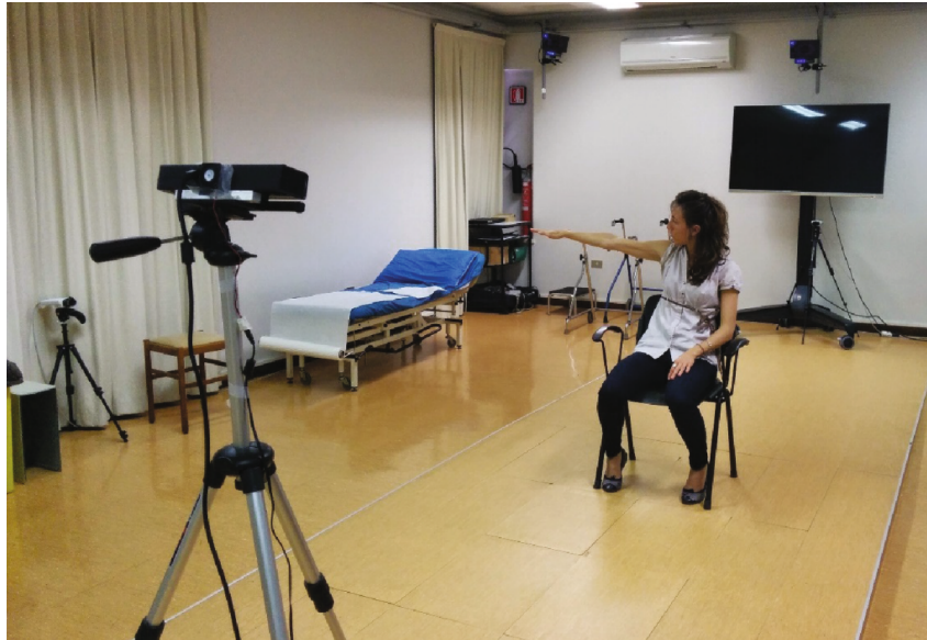
Figure 3 – Color-depth camera system used to track human motion (Source: Clark et al. (2019))
