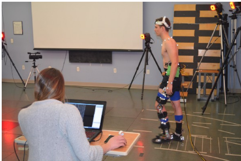
Figure 2 – Marker-based systems to track human motion (Source: Pfister et al. (2014)).
