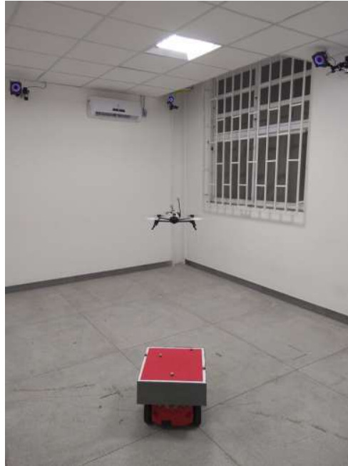
Figura 3 – Pioneer 3-DX and Bebop 2 with their OptiTrack markers and three of eight cameras
