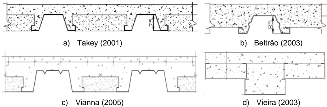
Figure 1.3 — Cross-sectional view of four different composite ribbed slabs.
