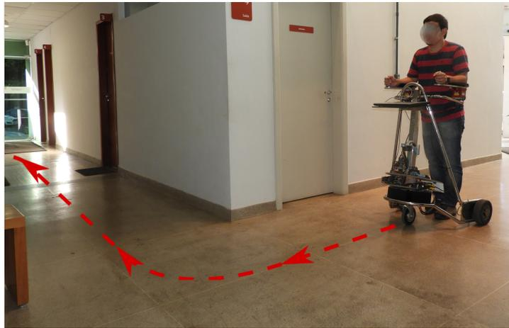
Figure 7 – Case study scenario: the smart walker guides user displacement inside a facility through automatically generated virtual trails. The interaction forces measured by the force sensors under the handlebars are used as inputs to control walker velocities.
