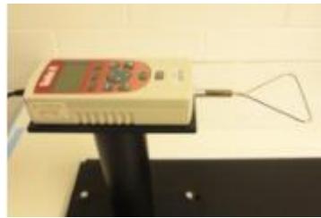
Figura 36: Medidor de força de agarre ( grip test ). (Fonte: https://www.robarts.ca/research/core_facilities/neurobehavioral_core_facility )
