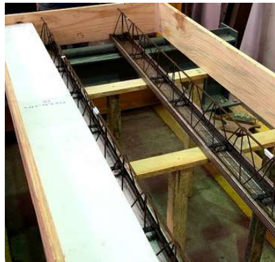
Figure A.3. (a) Weighting of slab components; (b) Assemblage under progress; (c) Assemblage completed. Source: Author.
