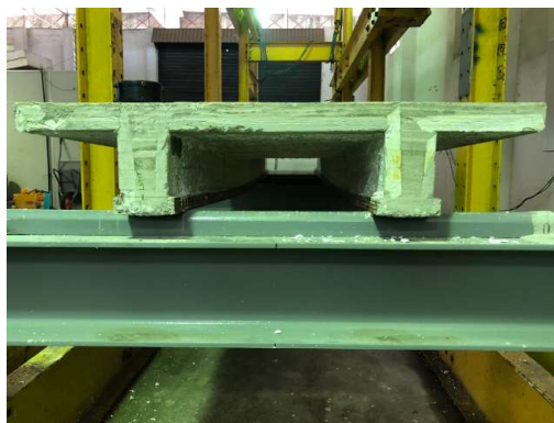
Figure A.18. Removal of light filling blocks to evidence the cracking patterns of composite slabs (TS2.5_16_0.33). Source: Author.
