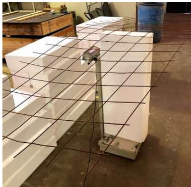
Figure A.3. (a) Weighting of slab components; (b) Assemblage under progress; (c) Assemblage completed. Source: Author.
