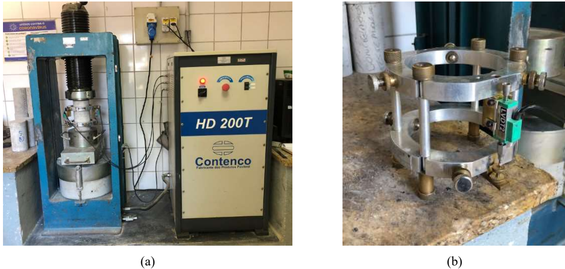
Figure 18. (a) Secant modulus of elasticity test; (b) Specimens after test.
