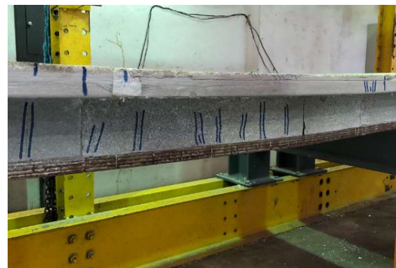
Figure A.18. Removal of light filling blocks to evidence the cracking patterns of composite slabs (TS2.5_16_0.33). Source: Author.
