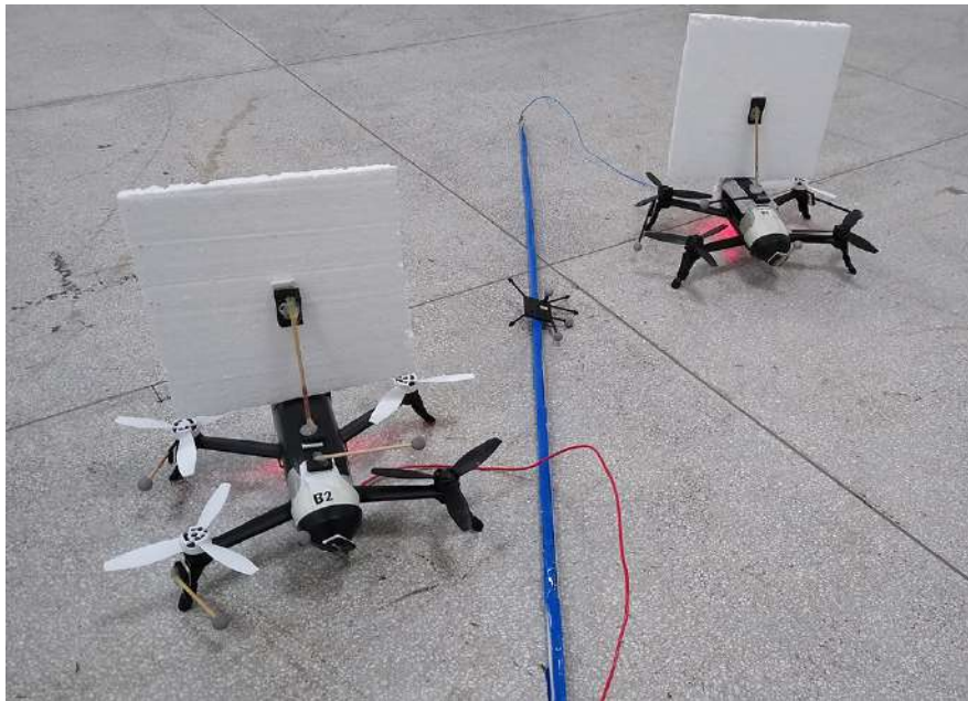
Figure 3.8 – Experimental setup containing the used quadrotors, bar-shaped payload, and drag foam plates.
