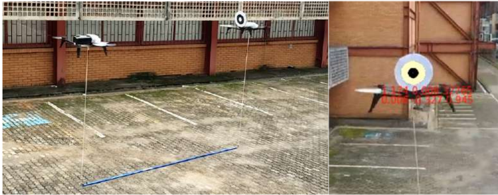
Figure 6.1 – The Parrot Bebop 2 quadrotors carrying the aluminum bar in outdoors using only onboard sensors and visual servoing.
