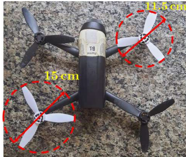
Figure 5.7 – A bebop 2 quadrotor with a damaged propeller.
