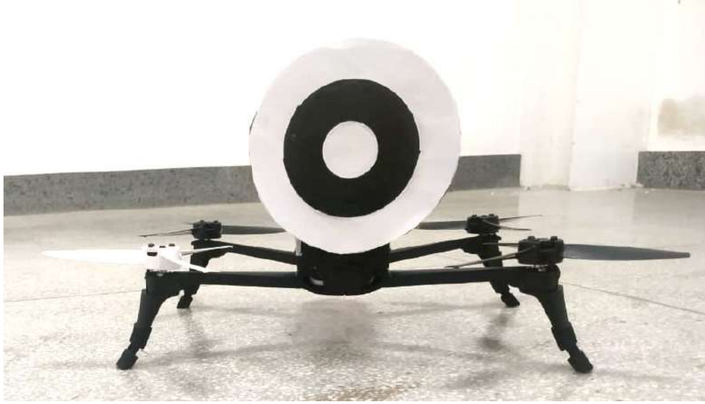
Figure 6.5 – Black and white pattern attached to the leader to be used by the follower to keep the desired distance t_{des} .
