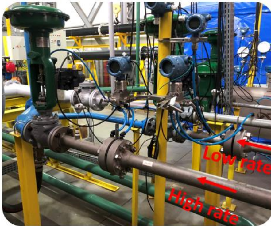
Figure 22 - The high and low mass flow rate orifice plate meters photography (Source: author)
