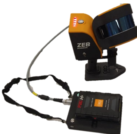
Figura 8 – LiDAR PLS GeoSLam ZEB-HORIZON 3D, modelo GS_510254.
