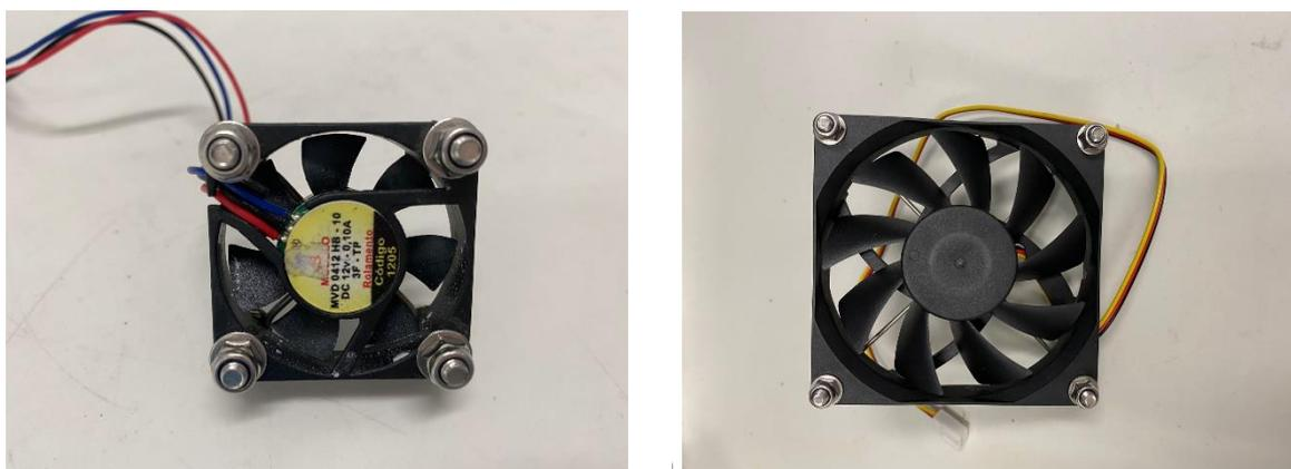
Figure 8 – Fans used at Flux hood. a) 4 x 4 cm in size, 6000 rpm and 12V and b) 8 x 8 cm, 3200 rpm and 12V.
