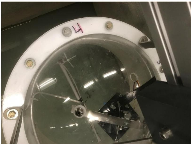
Figure 9 – Fan coupled and installed to a dome-shaped topper (view from dome-shaped topper outside).
