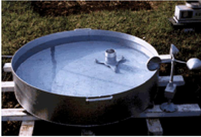
Figura 3-13: Tanque Classe “A”
