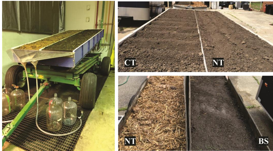
FIGURE 2 – Laboratory plots studied. CT - Contour tillage; DT - Downhill tillage; NT – No tillage; BS- Bare soil.
