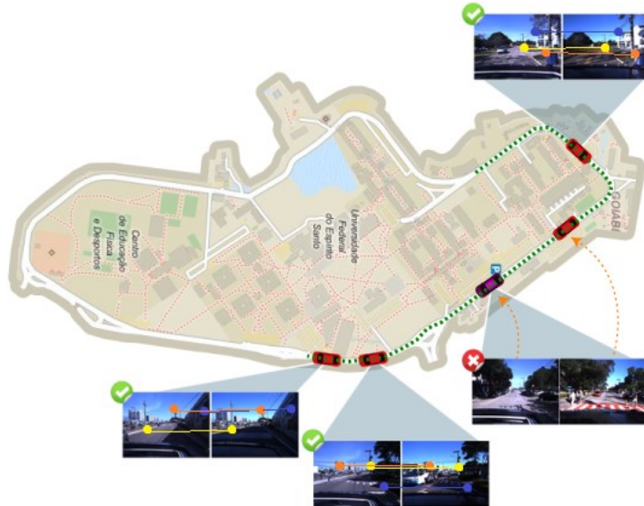
Figure 1.1: Illustration of VIBML performing global localization and position tracking around the UFES' campus. VIBML uses previously learned image-pose pairs stored in a neural map to estimate global poses (red cars) from currently observed images. VIBML's neural position tracking keeps a smooth trajectory (green dots), even in case of global localization failure (purple car).
