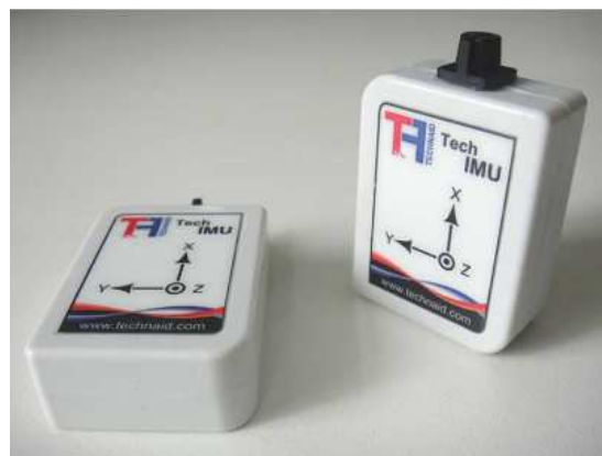
Figure 3.2 Tech IMU-CAN sensors, illustrating local coordinate systems. To describe the convention of the output of Technaid's sensors. (Source: MELIM, 2013).
