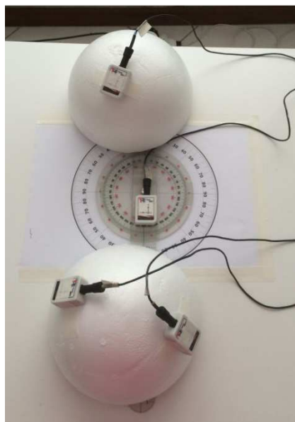
Figure 4.6 The two semi-sphere and goniometer set-up to explore the sensor-to-body segment calibration procedure.
