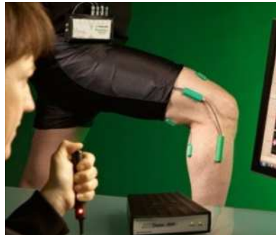
Figure 2.10 Flexible goniometer called SG150 for knee joint. (Source: BIOMETRICS, 2015).
