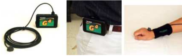
Figure 2.9 Polhemus G4 based on electromagnetic tracking system. (Source: Adapted from POLHEMUS, 2013).
