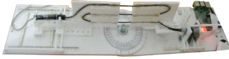
Figure 3.5: Side view of threefold-looped fiber measurement setup.
