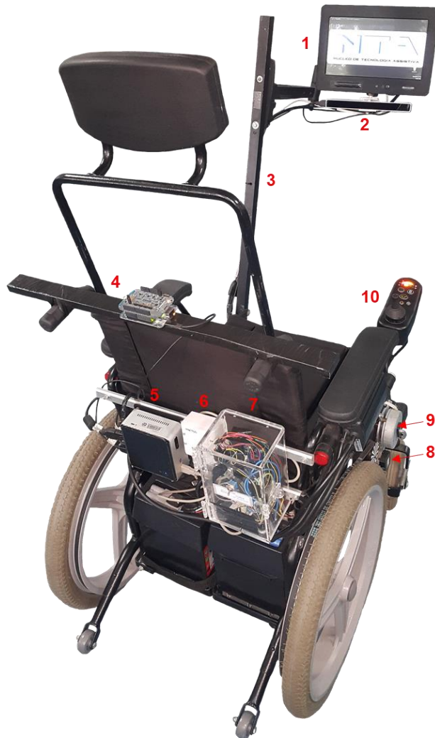
Fig. 7. Instrumented EPW used for tests in the RE and for the VE with Eye Tracker.
