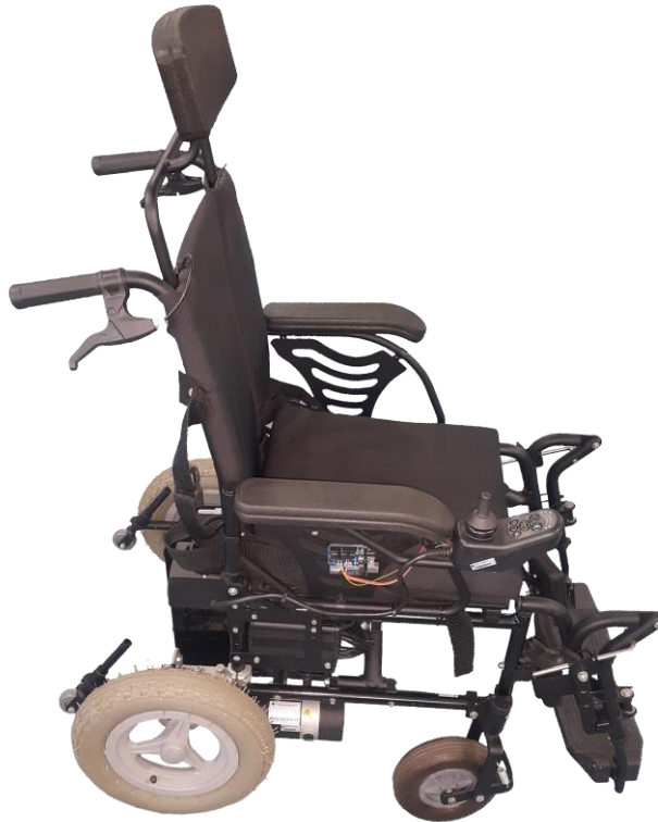
Fig. 4. Real Freedom EPW with no movement, where the user sits and uses the joystick as input for the Simcadrom.
