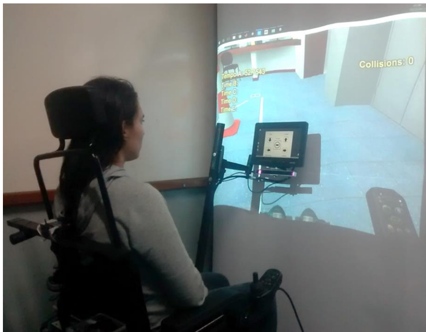
Fig. 6. A participant using the Simcadrom with eye tracker as an input interface.
