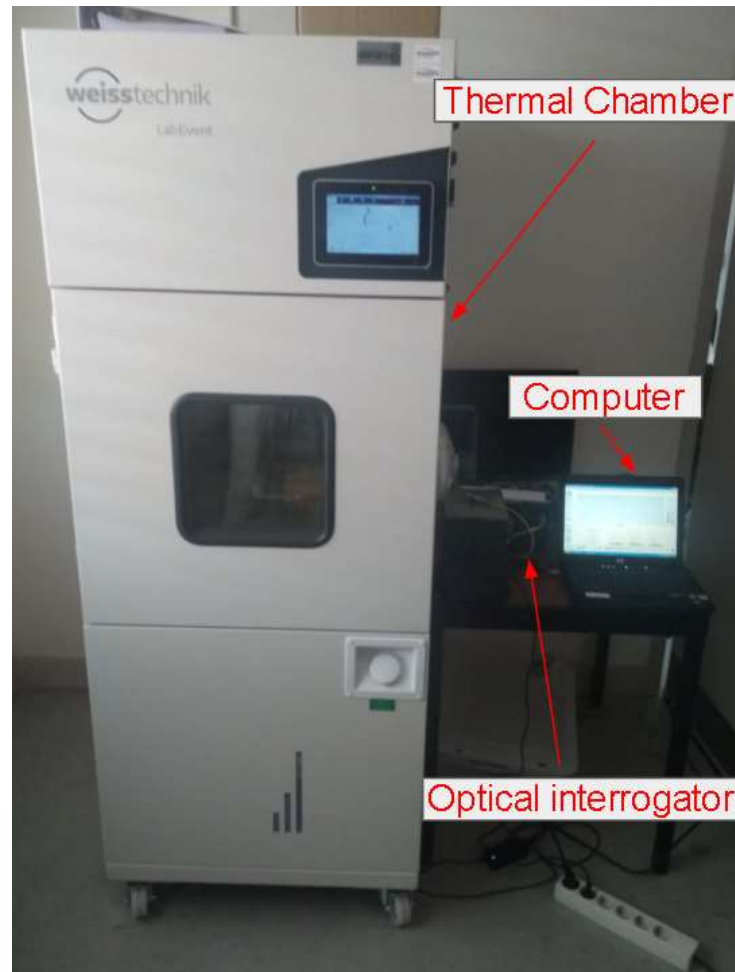
Figure 15 – Experimental setup for FBGs characterization to temperature variation.
