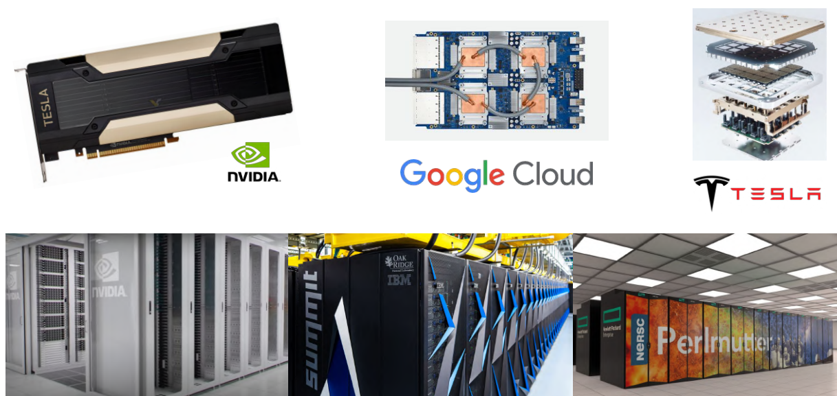
Figure 7 – Examples of accelerators (GPUs from NVIDIA, TPU from Google, and D1 from Tesla) and three of the fastest supercomputers with GPUs in the world (Selene from NVIDIA, Summit from ORNL, and Perlmutter from Berkeley).
