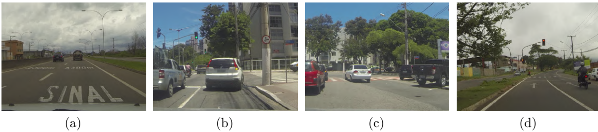
Figure 22 – Failure samples on the GOPRO dataset. The first two images are false positives, and the last two are false negative predictions. The second image is particularly difficult, because there is a crosswalk in the intersection and it does not fit into the criteria used for the manual annotation.
