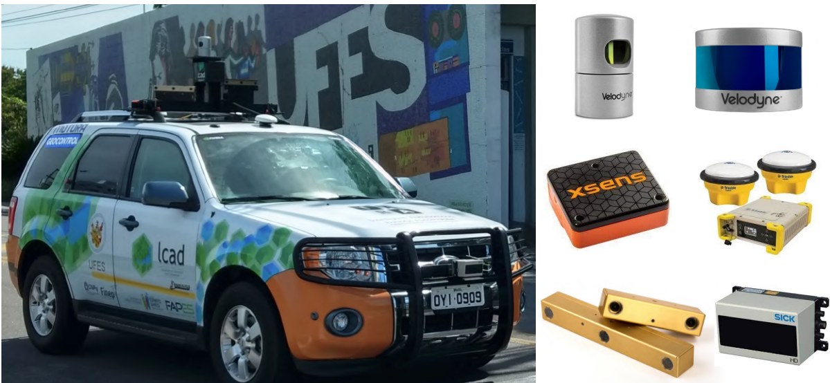
Figure 4 – Some of the resources that can be required to acquire useful data: vehicle, LiDAR, IMU, GPU, cameras, radar, etc.
