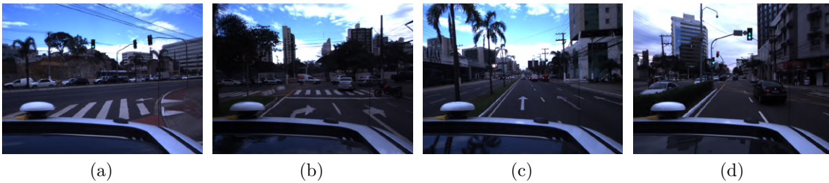
Figure 17 – Sample images of the IARA dataset. First two images are positive samples (contain crosswalks) and the last two are negative samples.
