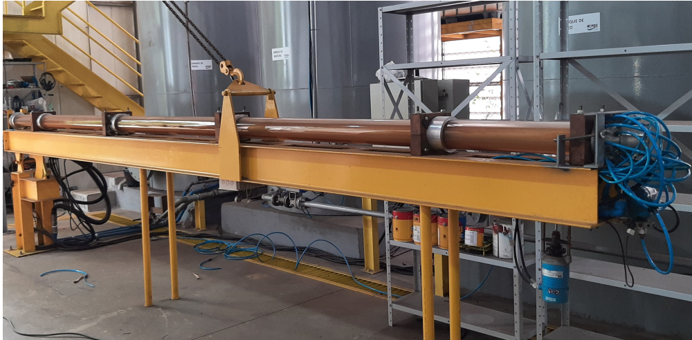
Figure 3 – ESP test facility - horizontal position
