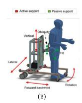
FIGURE 2.12: (A) Robotic platform with pelvic and body weight support on walking. (B) Robotic walker overview. Source: [73].
