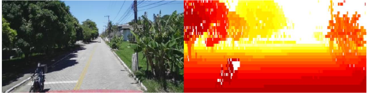
Figure 9. Comparison between camera image and LIDAR range image. The color scale in the image on the right represents LIDAR distance measurements that range from values close to zero (dark red) to 75 m (white) which is the defined limit of the scale.
