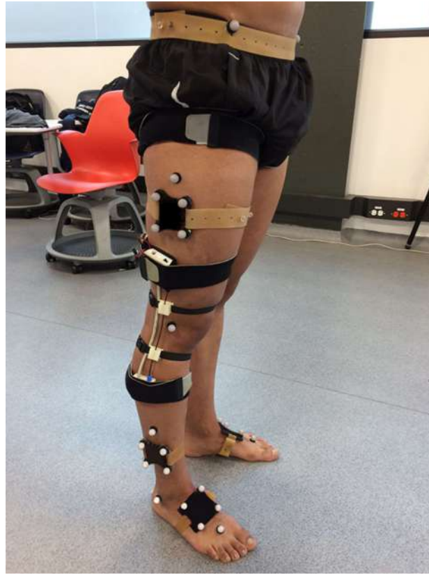
Figure 4.5: Marker set (Plug-in Gait lower body model), additional marker clusters and IMU-POF system placed on a participant.
